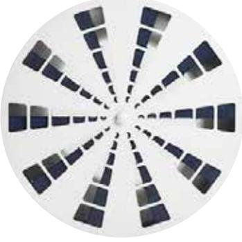
Ideal comfort diffuser electrically or manually adjustable diffusers are required for cooling and heating large halls. In order to prevent draughts in the cooling mode, the supply air must largely be discharged horizontally from the diffuser. It ensures optimum air distribution in cooling and heating modes.
