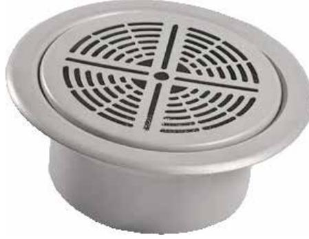
Floor Swirl diffuser is designed for use in raised access floor air distribution systems, where the floor cavity is used as a pressurised supply air plenum. The design achieves high induction rates of room air which optimises circulation and therefore comfort conditions.
